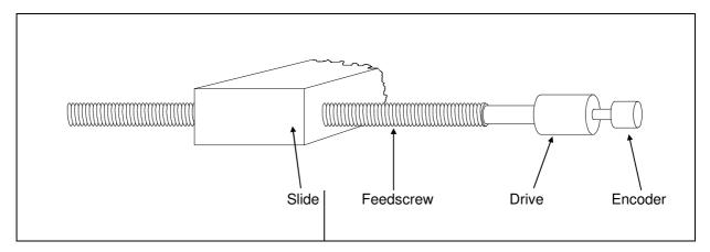
With Sinumerik Series 800 Control Systems, feedscrew errors can be largely compensated. For this purpose, the error curves of the machine axes are established by measurements with a laser interferometer setup. The "ZLM Position" program module determines the compensation values and transmits them to the machine control system.
